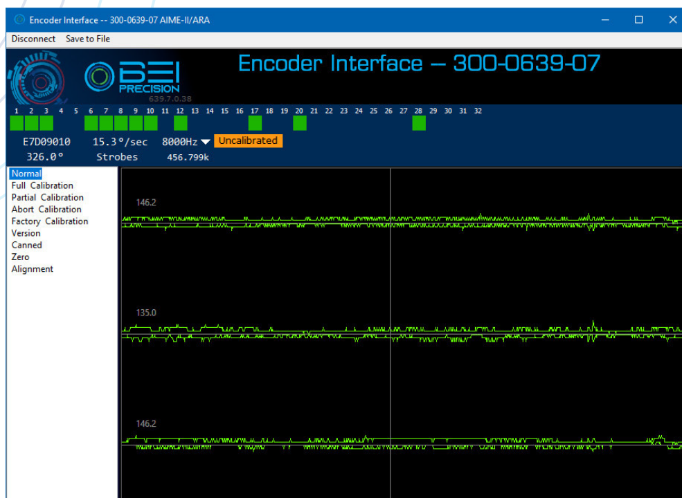
Figure 13: AIME-II Factory Calibration Command (same for ARA)
